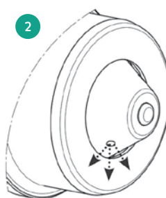
The residual pressure is released by the small holes during connection
